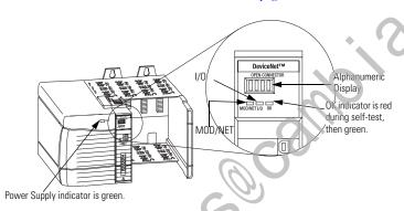
When you apply chassis power, the alpha numeric display cycles through the following information:
